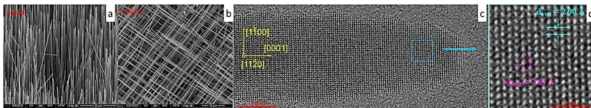
Figure 1 Vertically oriented ZnO nanowire on an a\text{-Al}_2\text{O}_3 [11\bar{2}0] substrate and at an angle of 60^\circ to an m\text{-Al}_2\text{O}_3 [10\bar{1}0] substrate; (c) HRTEM image of the ZnO NW tip with a diameter of approximately 10 nm; (d) magnified view of the frame from (c).
